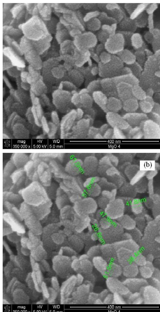
Fig.1: Shows the typical (a) low and (b) high-resolution FESEM images of nanoparticles obtained by the reaction of magnesium metal foil with water at 90°C for 9h.
