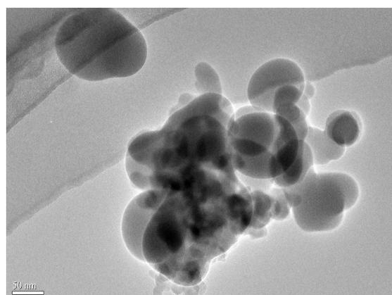
Fig.2: The TEM micrograph of MgO nanoparticle.
