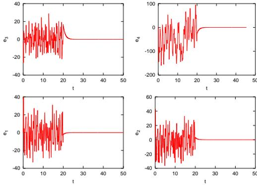
FIG. 2: Synchronization dynamics of identical hyperchaotic Lü systems. The controllers are activated at  $t \geq 20$
