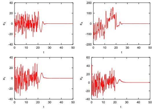
FIG. 7: Synchronization dynamics of hyperchaotic Lü and LS systems. The controllers are activated at  $t \geq 20$
