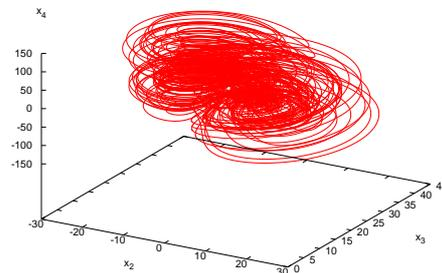
FIG. 1: Phase portrait of the chaotic attractor of the hyperchaotic Lü system with the following parameters  $\alpha = 36.0, \beta = 3.0, \gamma = 20.0$  and  $\eta = 1.0$ .
